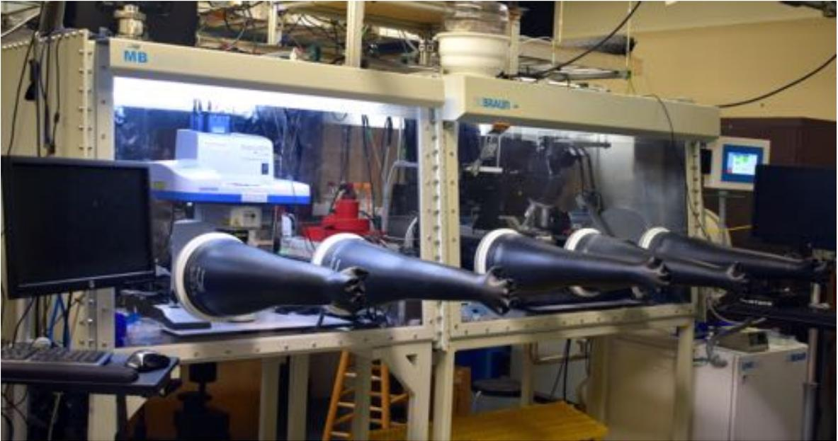
**Figure 4.6:** A nitrogen-filled glovebox at Columbia University used rigorously for fabricating the devices based on air-sensitive materials.
