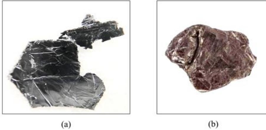
**Figure 4.1:** Bulk single crystals of (a) InSe bought from 2dSemiconductors (image from [www.2dsemiconductors.com/InSe](http://www.2dsemiconductors.com/InSe)). (b) GaSe bought from hq graphene (image from [www.hqgraphene.com/GaSe](http://www.hqgraphene.com/GaSe)).
